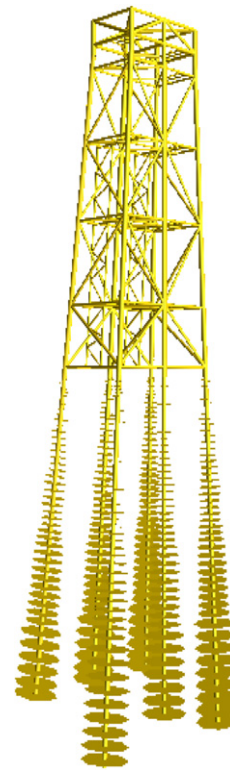
Fig. 2. Global view of the SPD2 platform, the jacket structure with piles.
