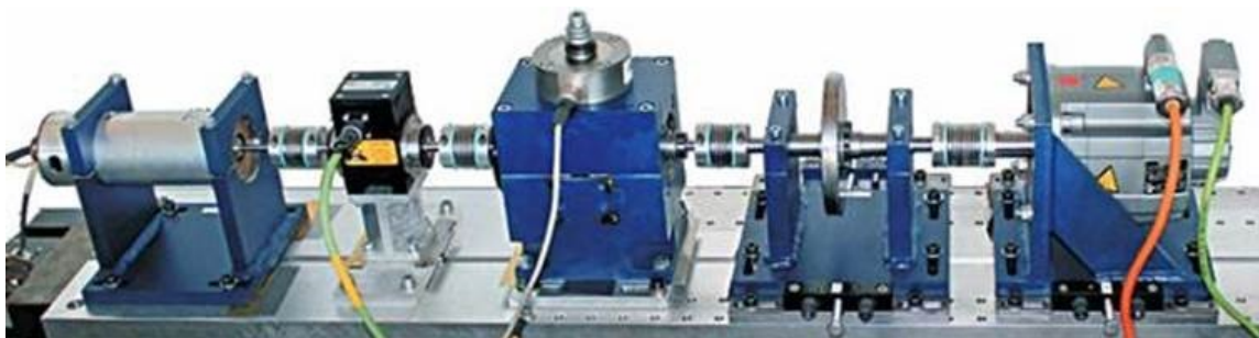
Figure 1: Mechanical structure of the test stand with test motor, measuring shaft, bearing module, flywheel, load motor (from left to right) [3].
