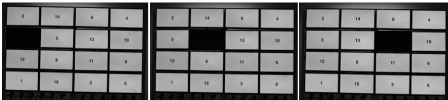
Figure 4.6. Distributed resolution of the N-puzzle on the wall of agentified screens. Each portion of the video represents a piece of data carried by a tile. The goal is to reconstruct the entirety of the video by displaying the numbers in the correct order
