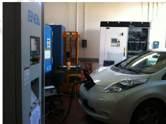
Fig. 2. The BESS inverted-controlled and the charge station during a test on a Nissan EV.
