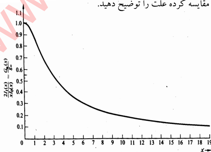
Fig. 4.5-6 Plot of 2I_1(x)/xI_0(x) vs. x .
